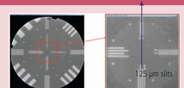
Figure 3. Resolution Test Pattern image obtained with an image plate fielded inside and outside the laser chamber demonstrating better than 0.125 mm resolution
