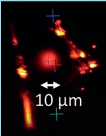
Emission from an X-ray heated warm dense plasma at Linac Coherent Light Source. The glowing circle is the emission from the plasma itself, and the jagged edges of the hole blown in the original gold foil are also illuminated by this emission. The cross-hairs are alignment fiducials from the camera used to take this image
