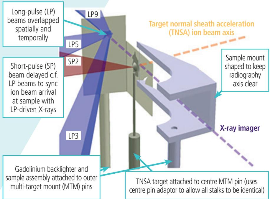
Schematic representation of the Orion experimental configuration
