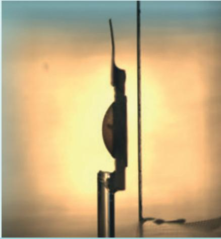
Side-on view of the Orion warm dense matter target, showing the gold hemisphere in position to focus an ion beam onto a single-crystal diamond ribbon. For scale, the ribbon is 20  $\mu\text{m}$  thick (approximately half the diameter of a human hair)
