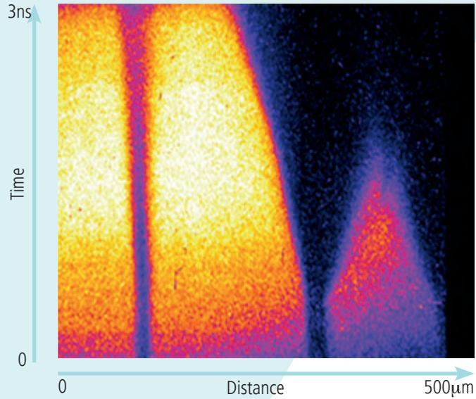
Streaked radiography of a target similar to the one shown above, showing the expansion of each component in time as it is heated. The space axis is essentially a projection of the middle of the target assembly
