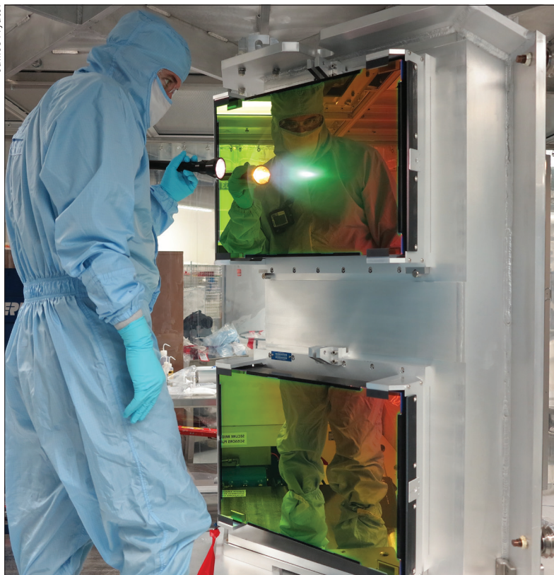
Final check Inspecting the cleanliness of mirrors for the Advanced Radiographic Capability – a petawatt-class laser currently under development at the National Ignition Facility.
