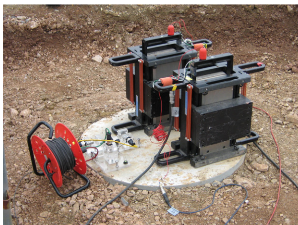
Figure 6. Shaker pile testing
