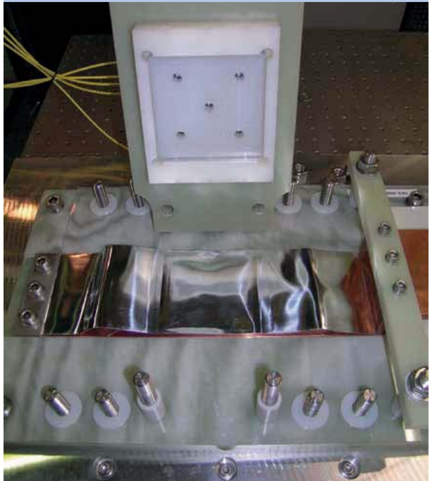
Foil flyer assembly – post firing.
