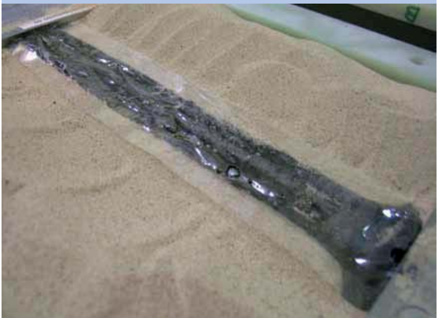
EFDR fuse after explosion.
