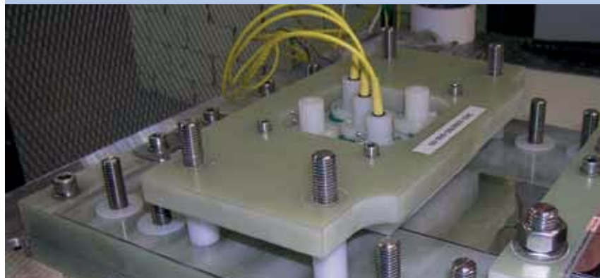
Foil flyer assembly – target holder in position.
