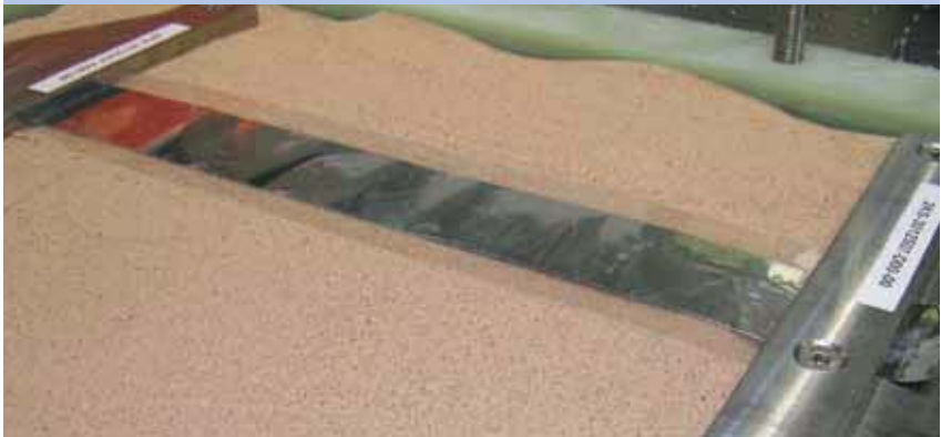
EFDR fuse before explosion.
